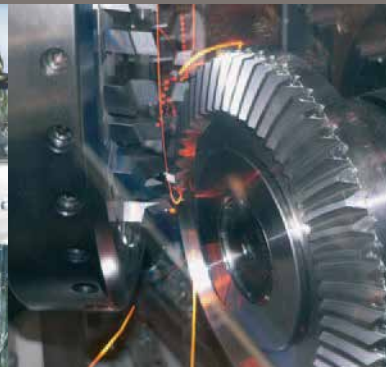
Dry cutting on spiral gear
